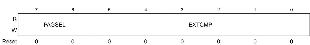
Figure 19-19. Debug Comparator B Extended Register (DBGCBX)
