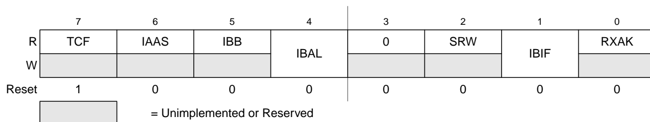
Figure 11-6. IIC Bus Status Register (IBSR)
