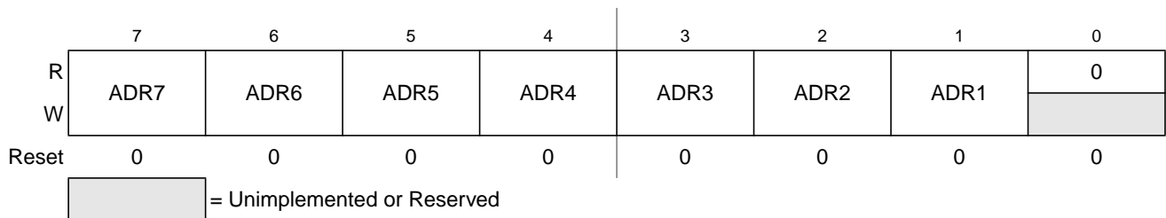
Figure 11-2. IIC Bus Address Register (IBAD)
