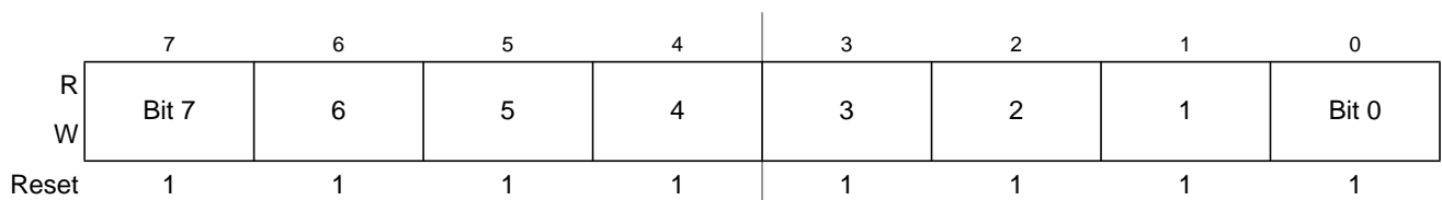
Figure 15-32. PWM Channel Duty Registers (PWMDTY5)
