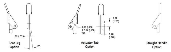
The bent leg option is required when using the extractor with Lok Tainers for PCB retention within sheet metal (non-cold wall) applications. Additionally, if using a lever actuated Lok Tainer, the actuator tab will work in conjunction with the lever to release the PCB.
