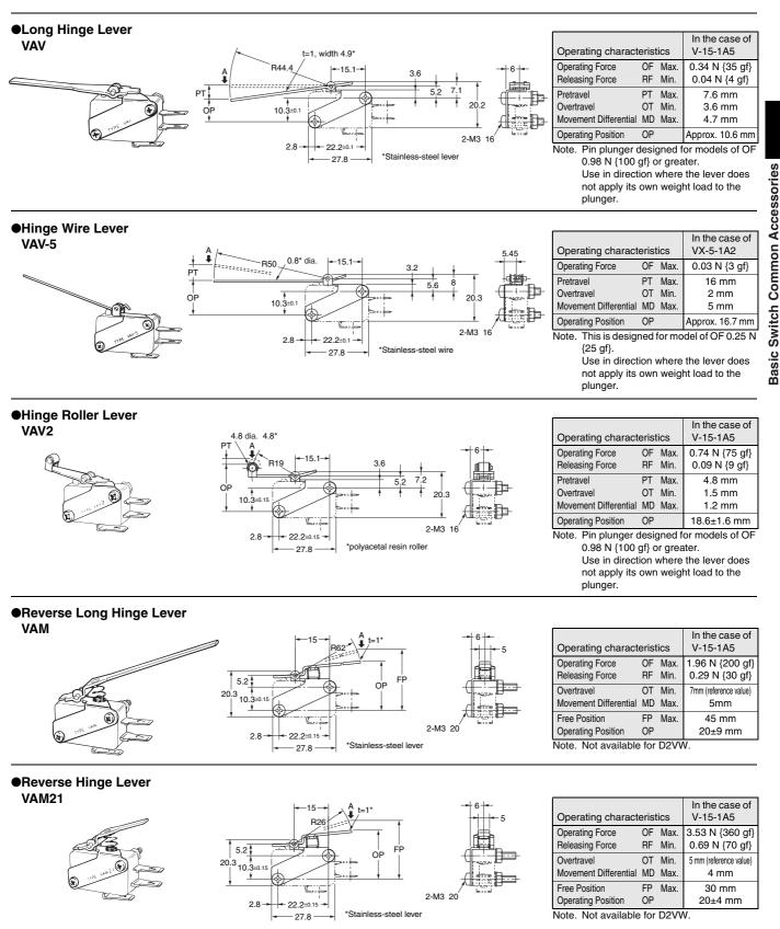
Note1. Unless otherwise specified, a tolerance of  $\pm 0.4$ mm applies to all dimensions. Note2. The operating characteristics are for operation in the A direction ( $\clubsuit$ ).
