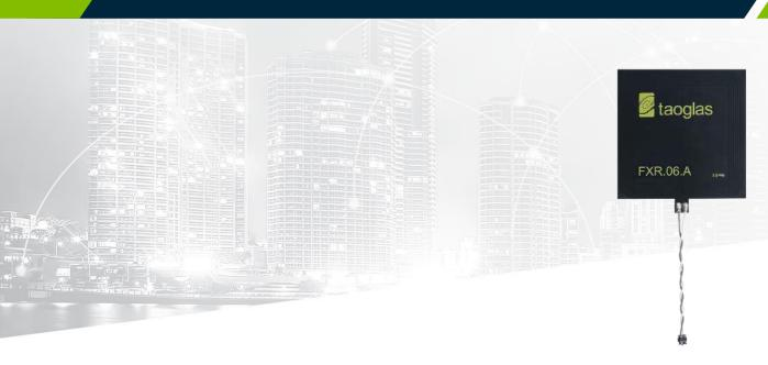
The FXR.06.52.0075X.A is a square, flexible, NFC (Near Field Communications) antenna for use in mobile devices and other applications such as keycards, payment systems, and boarding passes. The design provides a flexible NFC antenna with 75mm twisted pair 28AWG cable that can be adhered to the plastic enclosure of the device for ease of installation and work with specific 13.56MHz RFID and NFC chips which need to connect via JST ACH connector.
