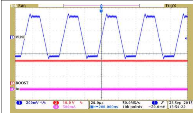
Figure 8-8. No Load, 22-kHz Tone Output
