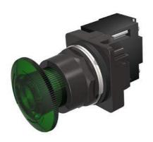
30mm BlackMax, Epoxy Coated Corrosion Resistant Metal Operator, Round Illuminated Twist-to-Release Full Voltage, 24V AC/DC LED Lamp Mushroom Head Cap Small 1.79" (45 mm) Plastic Cap, Green 2 Position Maintained, Twist-to-Release UL Listed, CSA Certified NEMA 1,3,3R,4,4X,12,13 & Automotive Standards
