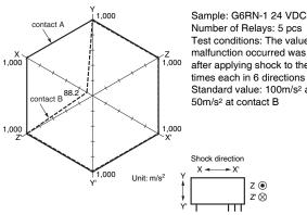
Number of Relays: 5 pcs Test conditions: The value at which malfunction occurred was measured after applying shock to the test piece 3 times each in 6 directions along 3 axes. Standard value: 100m/s<sup>2</sup> at contact A,
