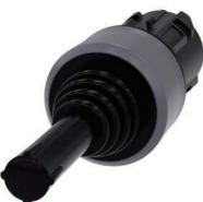
Coordinate switch, 22 mm, round, plastic with metal front ring, black, 2 switch positions, vertical, momentary contact type, without mechanical interlocking, with laser labeling, lower case
