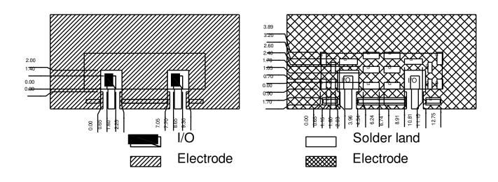
The recommended shielding case layout guide (min)
