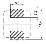
no sensitive traces underneath the component
