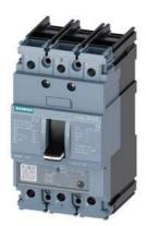
circuit breaker 3VA5 UL frame 125 breaking capacity class M 35kA @ 480 V 3-pole, line protection TM230, FTAM, In=80A overload protection Ir=80A fixed short-circuit protection li=5...10 x In cable connection on both sides
