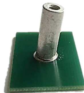
Test PCB for the Checking fixture Shearforce
