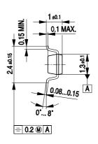
Note: Mold flash, protrusions or gate burrs of 0,2 mm max. per side are not included
