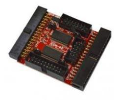
ICE40-DIO DIGITAL INPUT / OUTPUT BUFFER WITH PROGRAMMABLR VOLTAGE LEVELS FROM 1.65V UP TO 5.5V
