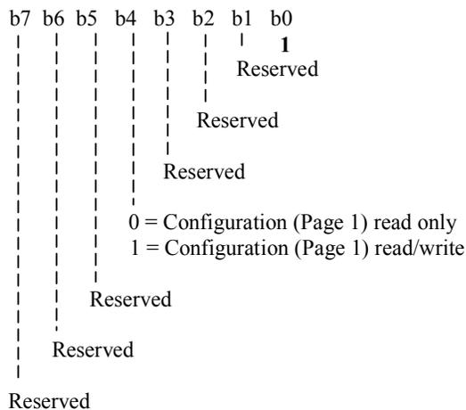
**Note that these configuration bits are OTP. Once they are set to read-only the Hitag 1 transponder is hardware protected and they can never be changed.**
