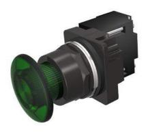
30mm BlackMax, Epoxy Coated Corrosion Resistant Complete Metal Unit Illuminated Push-Pull Operator Transformer type, 120V AC Incandescent Lamp Mushroom Head Cap Small 1 3/4" (44.5 mm) Plastic, Green 2 Position Maintained, Pull-to-Release UL Listed, CSA Certified NEMA 1,3,3R,4,4X,12,13 & Automotive Standards
