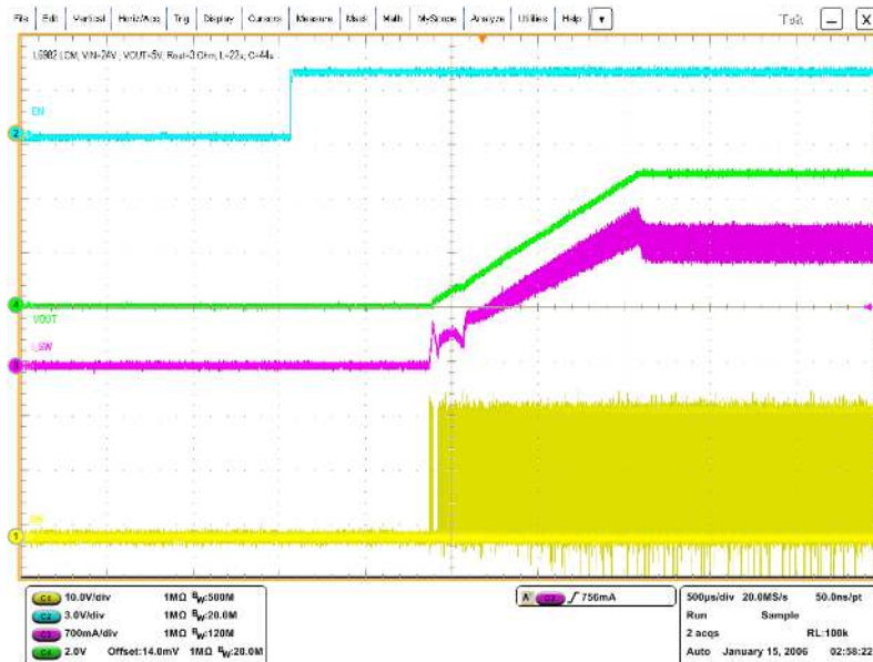
Figure 7. Soft-start phase with R_{OUT} = 3 \Omega
