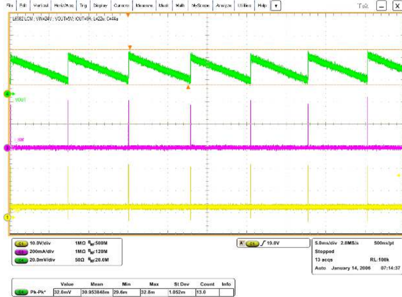
Figure 10. LCM operation over loading condition (part 1-pulse skipping)
