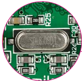
Figure 5-1: External crystal oscillator (X1)
