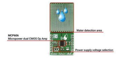
The MCP606 functions as a comparator on this click board<sup>TM</sup>.
