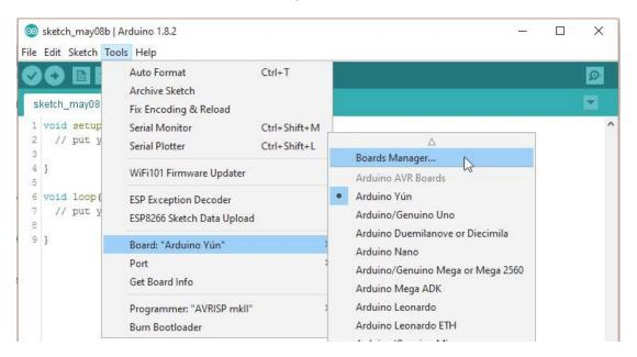
Once it loads, scroll down to the bottom, and you should see a listing for esp8266. Click on it, then on install, and install the latest version.
