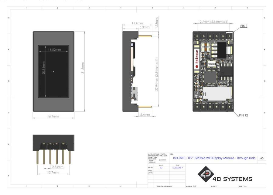
IoD-09 Series Mechanical Details - IoD-09-SM
