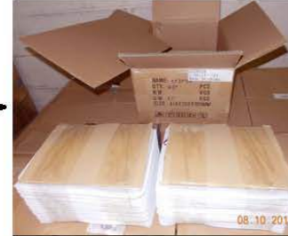
2 stacks of trays individually taped together in a bundle with layer of cardboard on top to protect the top layer of batteries
