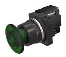
30mm BlackMax, Epoxy Coated Corrosion Resistant Complete Metal Unit Illuminated Push-Pull Operator Transformer type, 600V AC LED Lamp Mushroom Head Cap Small 1 3/4" (44.5 mm) Plastic, Green 3 Position Pull-Momentary/Push-Maintained UL Listed, CSA Certified NEMA 1,3,3R,4,4X,12,13 & Automotive Standards
