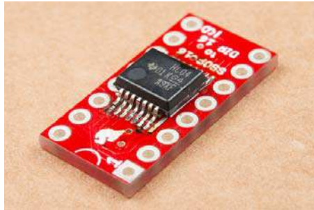
14 pins in a 16-pin adapter.
