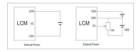
$V_{\text{DD}^{\sim}}V_{0}\text{: LCD}$  Driving voltage
