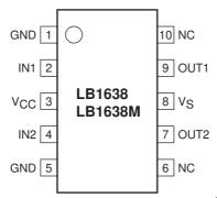
Note: both ground pins must be grounded.
