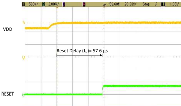
Figure 9-3. TLV840EVM RESET Time Delay ( t_D ) with No Capacitor
