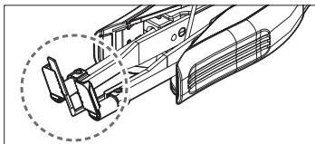
The lead adjuster can be removed with the handle cover attached to the handle.
