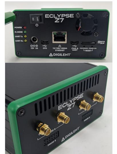
Screw the nuts back onto the SMA connectors.
