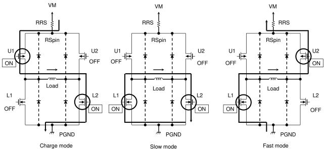
Charge mode A current flows into the motor coil.
