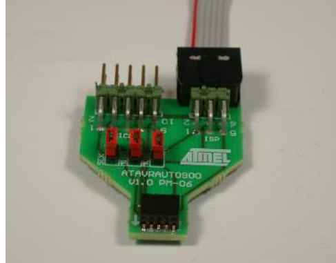
Programming the ATAVRAUTO102 using ATAVRAUTO 900
