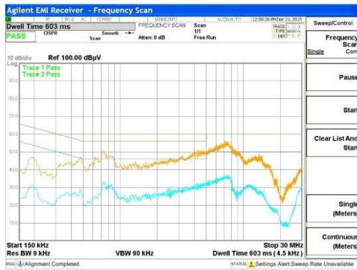
Figure 22. VIN = 115 V RMS , Load = 2.5 Ω
