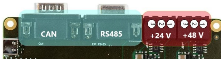
Figure 3: Power; Communication and USB-C connectors of TMCM-BB4
