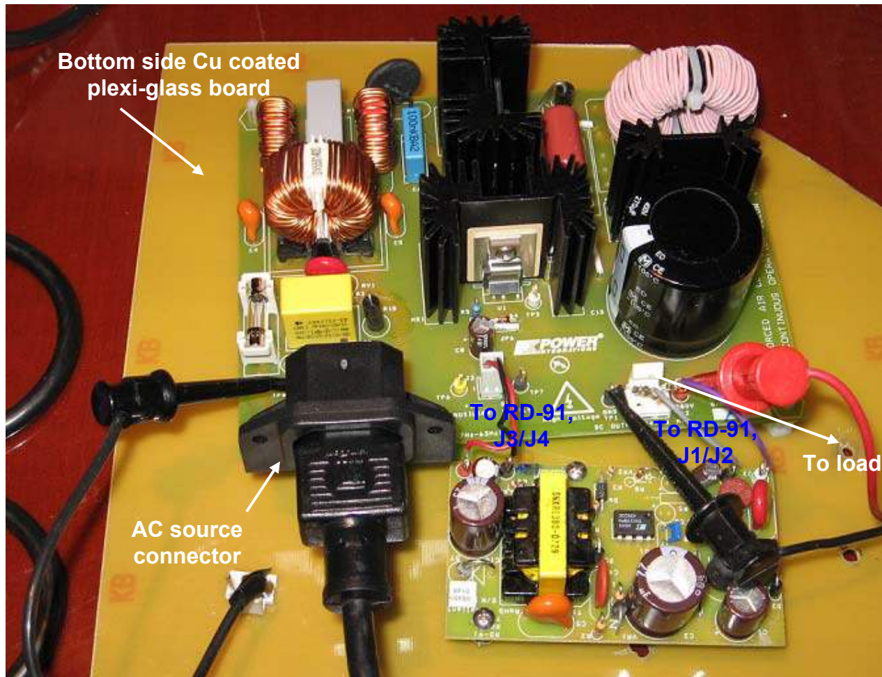
Figure 66 – EMI Test Set-up.
