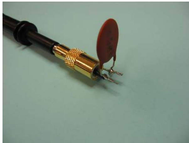
Figure 55 – Oscilloscope Probe with Probe Master ( www.probemaster.com ) 4987A BNC Adapter. Modified with wires for ripple measurement, and one parallel decoupling capacitor added.)
