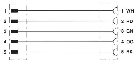
Contact assignment of 7/8" plug
