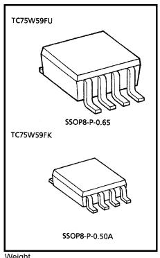
Weight SSOP8-P-0.65: 0.021g (typ.) SSOP8-P-0.50A: 0.01g (typ.)
