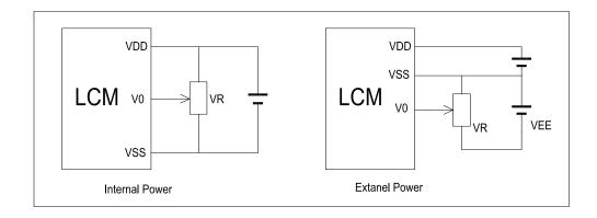
$V_{DD^{\sim}}V_0\text{: LCD Driving voltage}$
