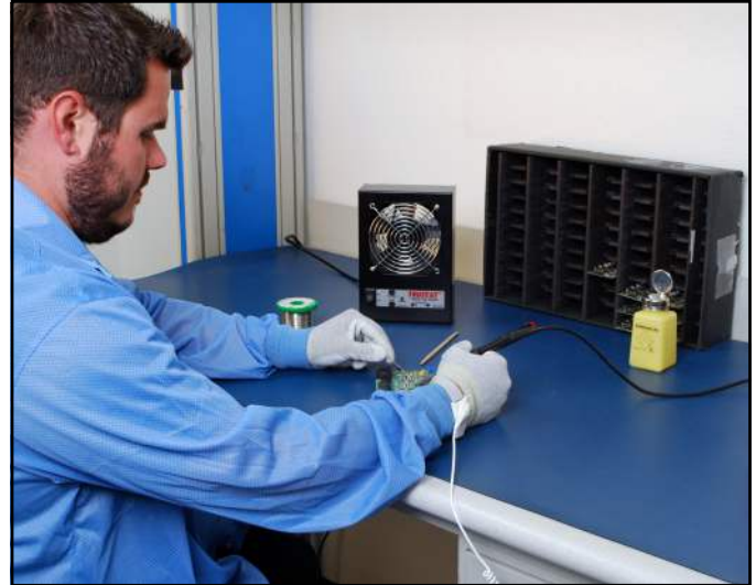
Figure 3. Using the Trustat Bench Top Ionizer at a workstation
