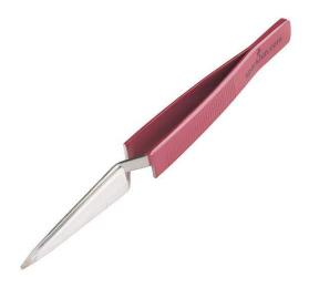
**Description:** These are nice, cross-locking, straight tweezers, unlike traditional models the tips on these tweezers will remain closed until squeezed open. They have a very fine tip which allows you to pick up very small parts with precision. This is a great tool to have if you're working with surface mount components or anything with very small parts. The ESD-safe coating will also help prevent electro-static damage to sensitive electronic components.
