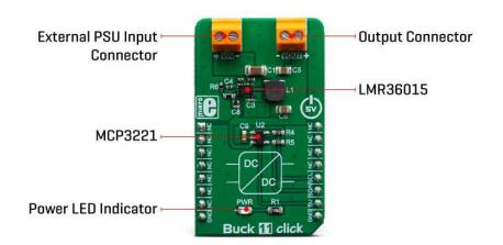
The output voltage is determined by the feedback voltage on the FB pin. The output voltage is set to 3.3V making it usable with most embedded applications, allowing them to be powered from the same source, like the rest of the application, which may use a higher voltage for its operation. This is a common-case scenario in various field applications where a relatively high voltage is required i.e. for servos, step motors, displays, etc.
