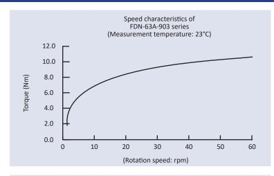
varies according to the rotation speed. In general, as shown in the graph to the left, the torque increases as the rotation speed increases, and the torque decreases as the rotation speed decreases. Torque at 20 rpm is shown in this document. In a closing lid, the rotation speed is slow when the lid begins to close, resulting in the generation of torque that is smaller than the rated torque.
