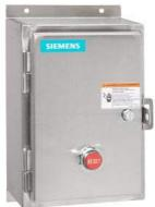
Non-reversing motor starter Size 2 1/2 Three phase full voltage Solid-state overload relay OLRelay amp range 25-100A 220-240/440-480VAC 60HZ coil Combination type Water/dust tight non-corrosive
