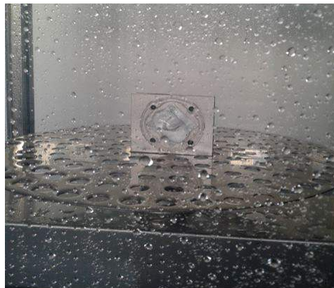
Testing under water jet
