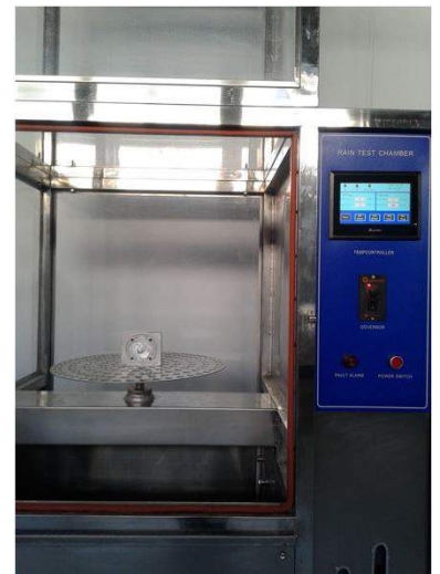
Testing under water jet
