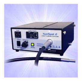
The SunSpot 2 is a next generation high-intensity compact light curing system. The unit was designed with low cost of ownership in mind, with its long-life UV/visible arc lamp, and filtered input long-life light guide. The SunSpot features easy to use exposure time controls and foot pedal activation. The system weighs a mere 6 pounds, and its 4 x 8.5 x 10.5 inch size is the smallest in its class.
