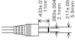
CLASS 2 POWER SUPPLY MODEL: WAU16-500 INPUT:120VAC 60Hz,11.2W OUTPUT: 16VAC @500mA
