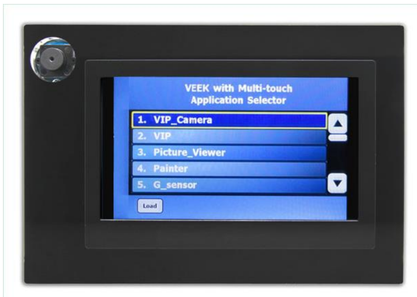
Figure 5-1 Application selector main interface
