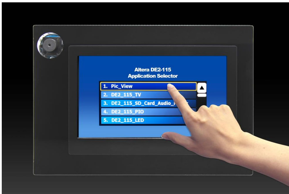
Figure 4-1 Application Selector Interface
