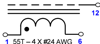
Figure 60 – Electrical Diagram, EE 41/33 PFC Choke.
