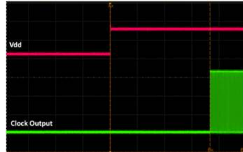
Figure 17. Startup Waveform vs. Vdd
