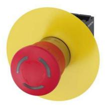
EMERGENCY STOP mushroom pushbutton, illuminable, 22 mm, round, metal, shiny, red, 40 mm, positive latching, according to DIN EN ISO 13850, rotate-to-unlatch, with yellow backing plate, without inscription, with holder, 1 NC, 1 NC, LED 24 V red, spring-loaded terminal, front plate mounting
