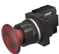
30mm BlackMax, Epoxy Coated Corrosion Resistant Complete Metal Unit Illuminated Push-Pull Operator Full Voltage, 120V AC/DC Incandescent Lamp Mushroom Head Cap Small 1 3/4" (44.5 mm) Plastic, Red 3 Position Pull-Momentary/Push-Maintained UL Listed, CSA Certified NEMA 1,3,3R,4,4X,12,13 & Automotive Standards
