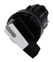
Selector switch, illuminable, 22 mm, round, plastic, white, selector switch, long, 2 switch positions O-I, latching, actuating angle 90°, 10:30h/13:30h, with laser labeling, upper case and lower case, always upper case at the beginning of the word
